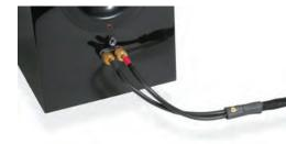
**Interconnect placement** - Place Carbon Tuning Disk on the cable, near the connector on the sending side of interconnects. Start at your source, and work toward your amplifiers, testing one color on both channels then the other on both channels.
