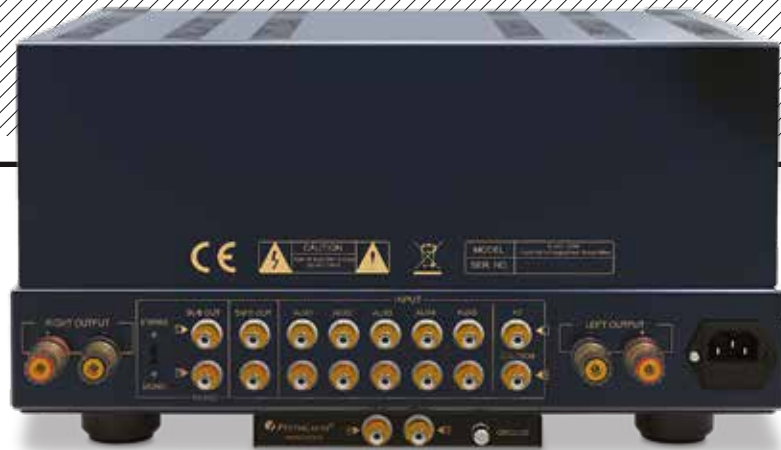
ABOVE: The EVO 300 Hybrid offers five line inputs, an HT bypass, tape out and sub/mono line outs with single 4mm speaker outputs configurable for stereo or (bridged) mono operation. Optional MM phono module also shown here
