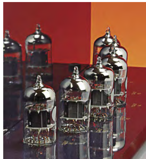
A rank of 12AU7 double triode small signal valves handle preamplification (2) and phase splitting/buffering (4).
