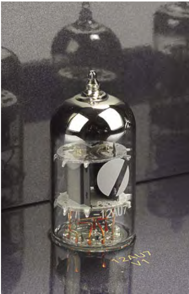
A 12AU7 double triode; six valves/twelve triodes in all are used. Typical life time is 10,000 hours and they are inexpensive.
