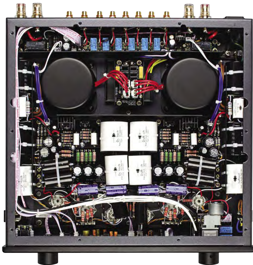
The inputs are selected by relays (top) and the two mains transformers for preamplifier are screened toroidals. There are specialised (white) capacitors and a motorised Alps volume control (bottom right).
