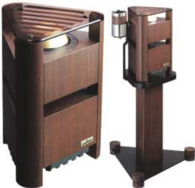
"The ES024 is a two-way speaker system consisting of a spherical ceramic squawker and a dynamic woofer. The squawker's spherical ceramic design offers excellent transient character and generates omni-directional spherical waves, providing superlative reproduction of the middle and upper ranges. Lower tones are produced by a sturdy, honeycomb vibration board that bounces the sound off the floor, generating omni-directional, rich and deeply impressive bass tones."
